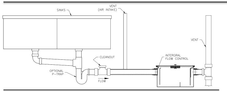
Zurn Grease Interceptors Z1170 consist of a interceptor rated at ( ) gpm and a properly sized intergal flow control.
