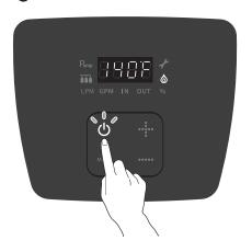
7 Touch the ":" button and the MODE button simultaneously for more than 5 seconds. "CAL1" appears on the digital display and start flashing.
