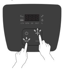
8 "CAL 1" flashes for about 6 minutes. When "CAL1" is flashing, it means the heat capacity is adjusting.
