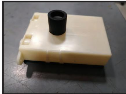
3. A 1/2" PVC coupling or bushing will fit snug over the 1/2" rubber hose. A 3/4" CPVC coupling or bushing will fit snug over the 5/8" rubber hose. This method ensures a water tight seal and also allows the condensate trap to be easily removed for service.
