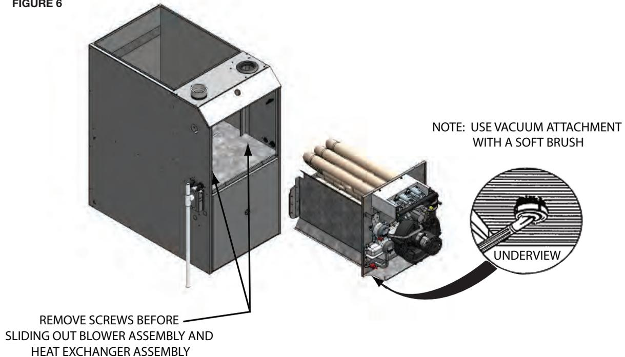
9. Once cleaning is complete, slide the heat exchanger back into its original position using the screw holes on the division panel for alignment.
