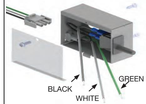
FIGURE 29 - INTEGRATED FURNACE IGNITION CONTROL
