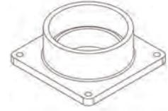
The combustion air inlet fitting is a 2” PVC Socket to Flange adapter. Install the adapter to the outside of the exterior panel using the screws provided (ensure gasket is properly placed between the adapter and the outside of the exterior panel for proper sealing). **Failure to apply gasket on cabinet exterior voids the warranty.**
