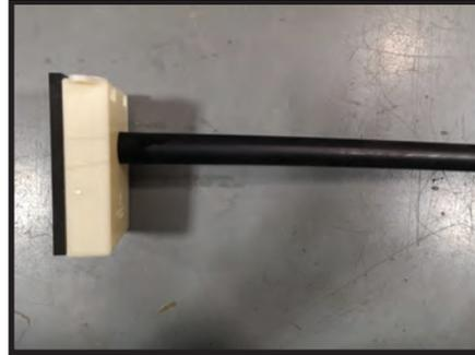
2. If installing with 1/2" PVC, use the 1/2" hose. If installing with 3/4" CPVC, use the 5/8" hose. Slide the appropriate hose over the condensate trap outlet and cut it flush with the end of the outlet. The remaining rubber should be flush with the end of the outlet on the condensate trap. The remaining hose is sufficient length to accommodate all furnace orientations.
