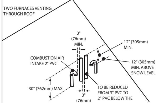
If more than two furnaces are being installed in close proximity, each additional combustion air intake and exhaust termination set shall not terminate less than 12 in (305mm) apart. Note: Canadian installations of 120000 Btu/hr require 3 ft (915mm).
