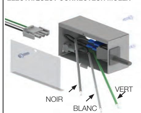
FIGURE 29 - CONTRÔLE D'ALLUMAGE DE FOURNAISE INTÉGRÉ
