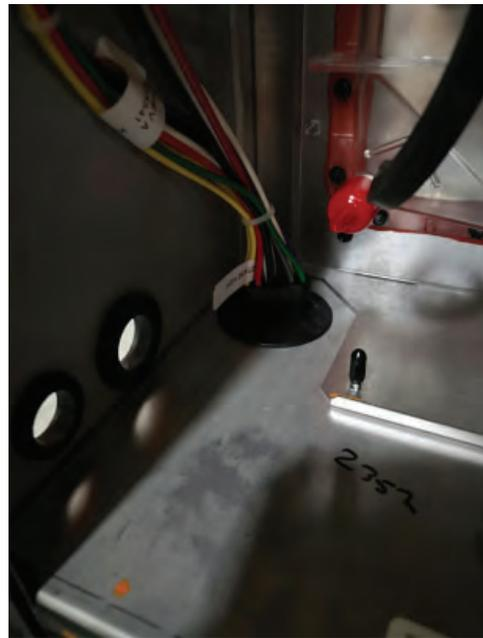
7. Pull the heat exchanger assembly out.
