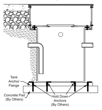
Tank Anchor Flanges are welded to the tank bottom and supplied with holes for hold down anchors (By Others) to attach to a concrete pad. Tank Anchor Flanges are recommended for securing the tank to the ground in partially full or high water table tank applications.
