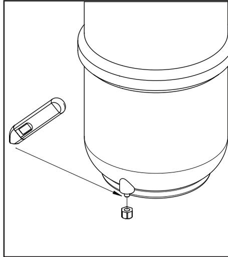
1. Turn off water supply to your RO system by turning off the adapter valve. Open the faucet to drain the storage tank.
