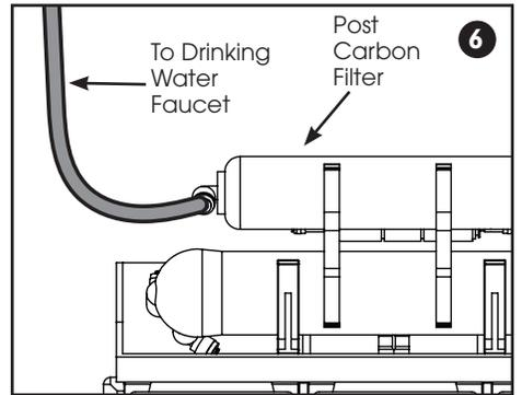
6. Attach Tubing to Post Carbon Filter
