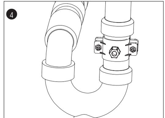
4. Attach 1/4" tube by slipping the tube through the black compression nut and hand tighten the nut on to the saddle valve.
