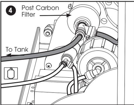
4. Attach 3/8" Tubing to Post Carbon Filter
