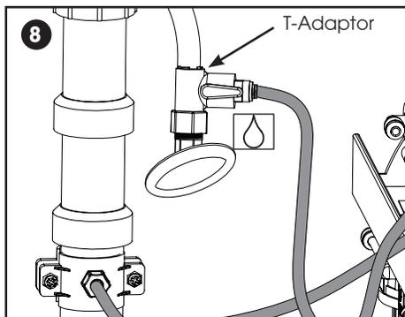
8. Connect Tubing from T-Adaptor to RO Inlet
