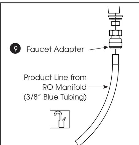
3. Take another length of 3/8" tubing and make sure it is has a fresh cut and is free of foreign materials and any scratches on the outside surface. Install the tubing into the push in type fitting at the base of the faucet. Make certain that it is inserted all the way in; once inserted give it a slight pull to make sure it is locked into the fitting. You have now completed the tubing connections.
