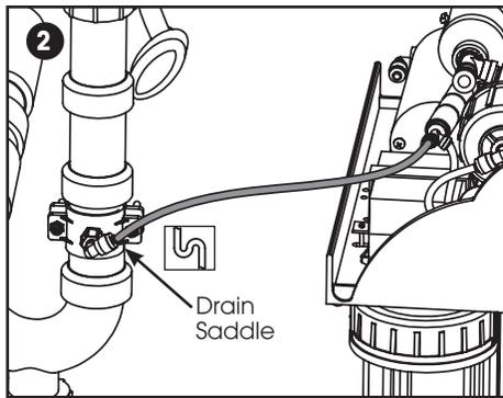
2. Attach the other end of the 1/4" tubing to the drain saddle
