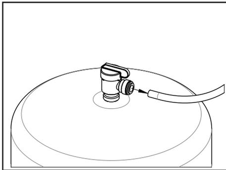
1. Turn off water supply to your RO system by turning off the adapter valve. Open the faucet to drain the storage tank.
