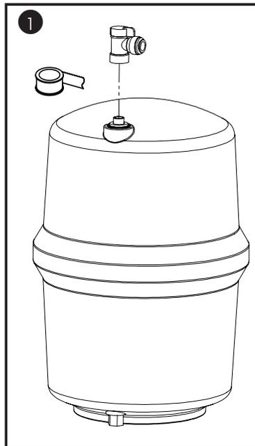
1. Apply teflon (PTFE) tape to threaded fitting at top of tank. Wrap tape around clockwise 3 to 6 times for a good seal. Attach Shutoff valve
