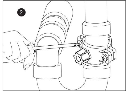
2. Tighten the clamps with the help of the two bolts.
