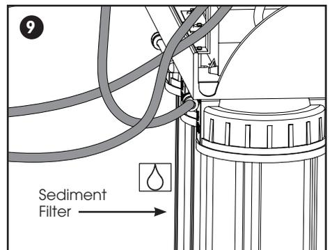
9. Connect Tubing from T-Adaptor to RO Inlet
