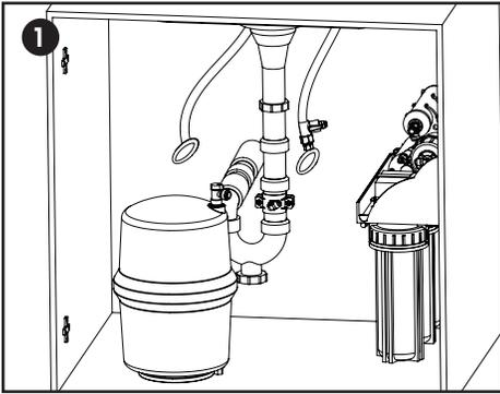
1. Place Tank under the sink. The Shut off valve is already installed in the early steps
