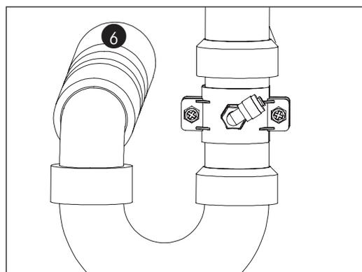
In case of airgap faucet install the elbow fitting and install the 3/8" Tubing
