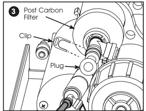
3. Remove Blue Clip and plug from Post Carbon Filter
