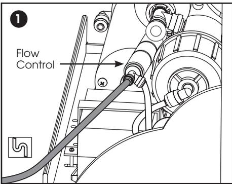
1. Attach 1/4" Tubing to Flow Control
