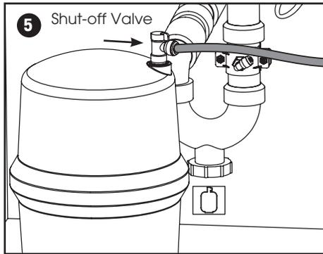
5. Attach Tubing to Tank Shut-off Valve
