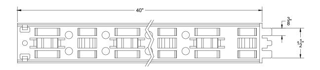
QuadRails $^{\text{\tiny{M}}}$  may require additional fasteners, such as foam-board staples or plastic nails to secure the rail to the subgrade or insulation boards. Additional fasteners are not included with the QuadRail $^{\text{\tiny{M}}}$ .
