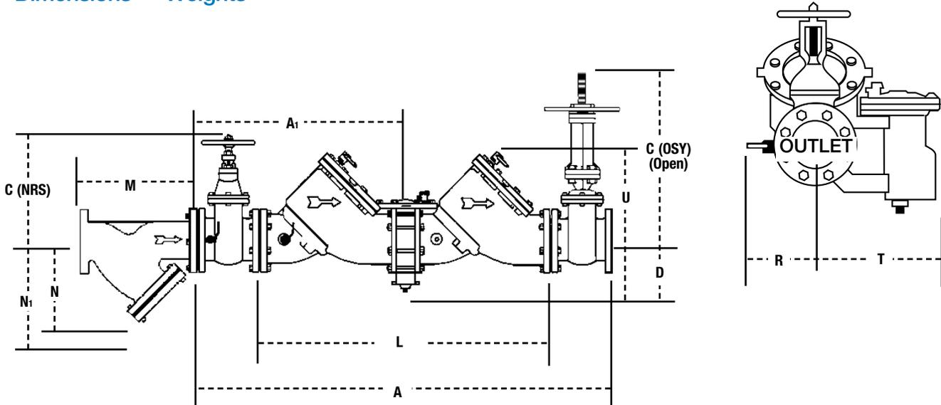
Note: Relief valve section is reversible, therefore, can be on either side and is furnished standardly as shown.
