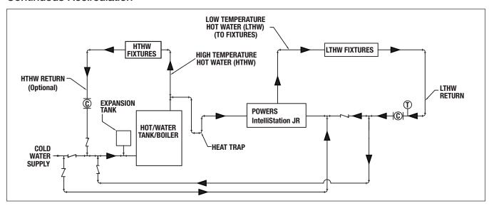
© Select flow rate as necessary to ensure Powers IntelliStation JR is operating at an ASSE 1017 minimum certified flowrate. See Literature.
