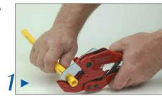
Wipe with a clean dry cloth. Inspect for scratches or gouges. If any, cut again so that the last 2 to 6 inch section, depending on size, has no surface defects.
