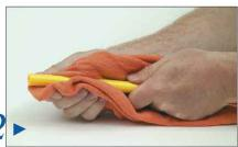
Use the Perfection chamfering tool for a proper O.D. chamfer. This chamfer permits the tube to be completely stabbed
