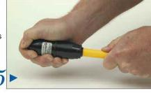
sizes through 1-1/4" CTS, and approximately 3/8" on the 1-1/4" and 2" IPS sizes. The tube must bottom out in the fitting. Pressure test the joint in accordance with your standard procedures. The reference mark can move outward up to an additional 3/8" during pressure testing.
