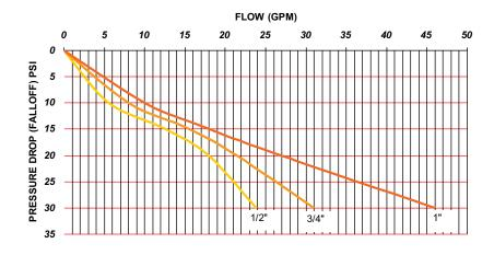
Note: Flow curves are based on static conditions of 100psi inlet pressure and 50 psi outlet pressure. Pressure differential is the difference between the supply pressure and adjusted outlet pressure measured in the static (closed) condition.
