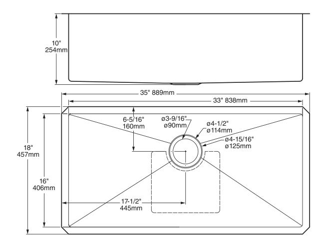
NOTES: \* DIMENSIONS SHOWN FOR LOCATION OF SUPPLIED AND "P" TRAP ARE SUGGESTED. FITTINGS NOT INCLUDED WITH FIXTURE AND MUST BE ORDERED SEPARATELY. SEALING COMPOUND SUPPLIED BY OTHERS.
