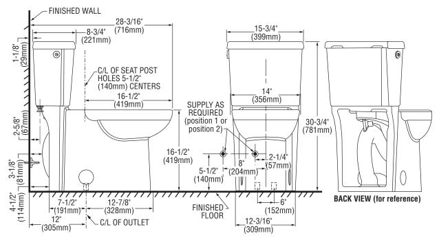
IMPORTANT: Water supply on the wall is required at 2-1/4" or 8" from centerline of the toilet (see rough-in). First suggested position is hidden behind the toilet. The geometry of the toilet gives space for this installation. The second suggested position is next to the toilet. Between these two positions, the space for the supply between wall and toilet is limited to 4-1/2". In this case, check your supply and hose dimensions.
