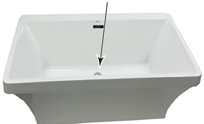
3. To disassemble the bathing well from the apron of the bathtub, invert the tub. Using a screw driver or drill, remove the 4 screws holding the 2 tub pieces together.
