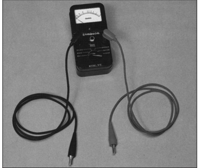
The Ohmmeter is used for measuring the electrical resistance of a wire circuit. The unit of measurement is called an Ohm.
