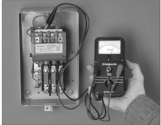
**⚠ WARNING** Open master breaker and disconnect all leads from starter to avoid damage to meter or electric shock hazard. Connect the ohmmeter leads as shown above.
