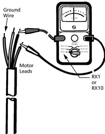
by 0.61 to determine the actual resistance of aluminum cable.
