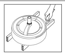
After checking fit and alignment, turn sink upside down and apply a generous portion of sealant around the under side of the rim near the edge.
