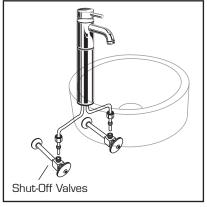
Connect supply line to faucet (finger tight) and carefully bend tubes to engage with the supply shut-off valves. Tighten connections at faucet and shut-off valves for secure seal.
