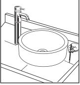
Before applying the sealant, place the sink temporarily into the cut-out. Check for alignment and clearance. Then mark the sink *and* countertop in several places as a guide for the installation location.
