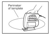
Cut opening around the perimeter of the template.
