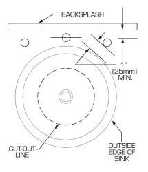
Drill a clearance hole inside the perimeter line of the template.
