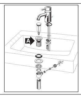
Mount the faucet and drain assembly (not included) on the sink or on the countertop following the manufacturer's instructions. Be certain to apply a bead of sealing putty on the underside of the drain (Part "A") in order to ensure a watertight seal between the sink and drain. Remove excess putty after installing drain on sink.
