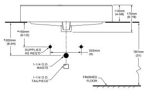
NOTES:  $\star$ DIMENSIONS SHOWN FOR LOCATION OF SUPPLIES AND "P" TRAP ARE SUGGESTED. FAUCETS NOT INCLUDED WITH FIXTURE AND MUST BE ORDERED SEPARATELY. FOR COUNTERTOP CUTOUT AND INSTALLATION INSTRUCTIONS USE TEMPLATE SUPPLIED WITH SINK.
