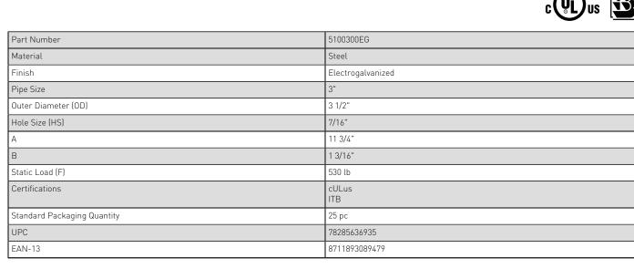
Clamp is fitted for steel pipe and should be installed below a coupling or shear lug, with bolts torqued to recommended value. Slotted holes and bolts for pipe sizes up to 12" only.
