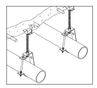
Continuous concrete inserts, installed in the ceiling, can be used to support trapeze hangers, suspended pipe racks, cable trays and single or multiple pipe hangers.
