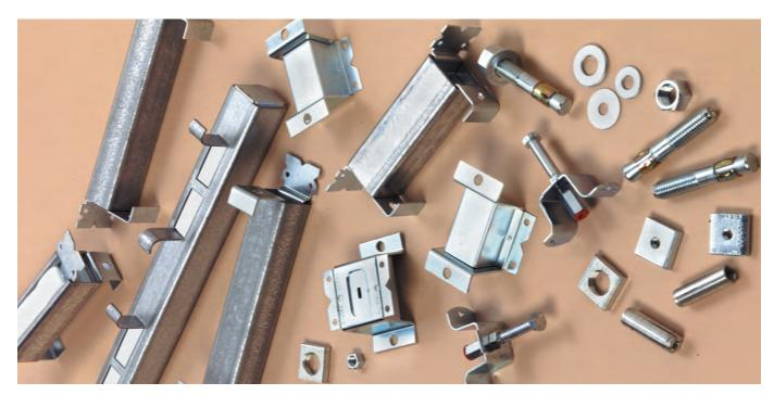
Continuous slot concrete inserts are designed to provide a pre-set support system cast in concrete ceilings, walls, and floors to allow flexibility of attachment at any point along the channel. This provides an excellent support system for pipe, conduit, and cable trays.
