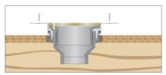
Blocking up a standard drain (with wood or strut) from The Halo installs easily from the top side of the floor. Cut a 6" hole and secure with screws or nails.
