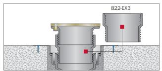
**Extension Adapter:** The 822-EX3 extension adapter installs between the Halo base and the head adapter. Stack multiple adapters if needed.
