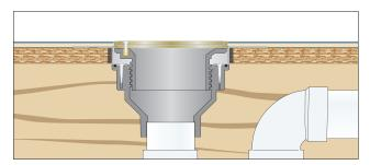
Minimal adjustment needed for thin flooring. Most 2" traps will fit in a 10" joist cavity.
