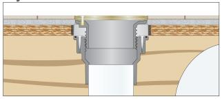
Head adjusts up to 3/4" for thicker flooring. Most 3" traps will fit in a 12" joist cavity.
