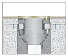
Remove the Coring Plug and replace with the Finish Fixture. The Finish Fixture can be adjusted up to another 1" after the secondary pour.
