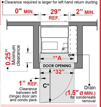
\* 32" x C (32.5") unobstructed clearance is required in front of the unit for complete removal of heating and cooling module.
