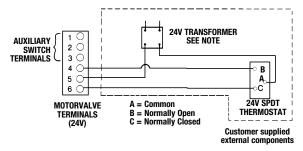
NOTE:  $1\!\!\!/4^u$  -  $1\!\!\!/2^u$  EMVII-6400SS-24-40 will operate with a 40 VA transformer. Thermostat must be capable of handling amp rating at stall.
