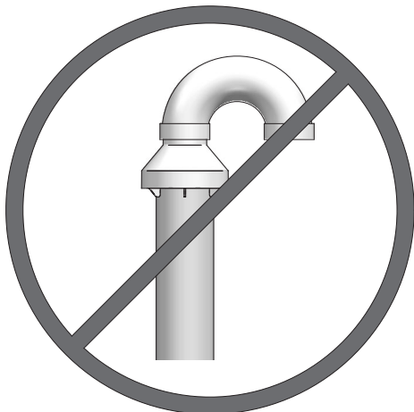
Figure 5-5 Do Not Install U-Bend to Rain Cap
