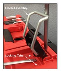
As an aid to removing a damaged Latch Assembly, use two large flat blade screwdrivers. Push blades between parts as shown. Twist both screwdrivers at same time to force the blades into opening and work the latch assembly over the two locking tabs.
