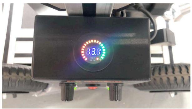
To work this correctly you must plug in all plugs on the machine and turn the switch on the front of the Control Panel to ON. Both Left Wheel and Right Wheel dials must be set at 0 MPH to get a true and accurate reading of how much battery power it remaining.
