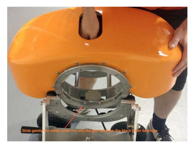
To remove the Head section from the Trolley Frame section gently lift the Head section out and upwards out of the roller bearings on the Trolley Frame section using the handle in the Head section. This should be easy to execute without considerable force.
