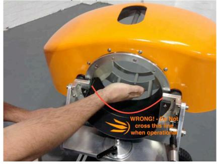
When in operation, inside the Head section of Ball Launcher is a distinct danger zone due to the firing wheels being capable to spin in excess of 3300 RPM. You must take great care that no part of your body, or anyone else present enters inside the Head section or touches the firing wheels when the machine is operational.
