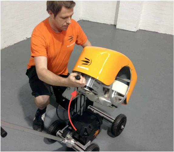
It is perfectly safe to rotate the Head section when operational or move any other of the handles when operational. This is why Ball Launcher can rapidly replicate many different deliveries from grass roots to professional level in quick succession.
