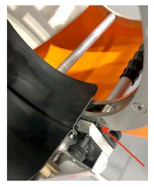
Please note that you must never try and remove the Head section from the machine when the Plunger Pin is in this position. It is locked into position and therefore you will not be able to remove it without putting the Plunger Pin into the fixed 'out' position.
