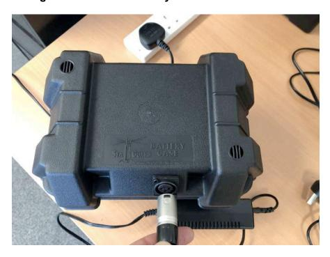
Typically the battery will take up to 4 hours to charge to 95% and will go onto a slower safety charge between 4 and 8 hours. It is fine to use the battery after 4 hours charge. Once charged, you will then be in a position to place The Battery Box in the holding section on the Trolley Frame section.
