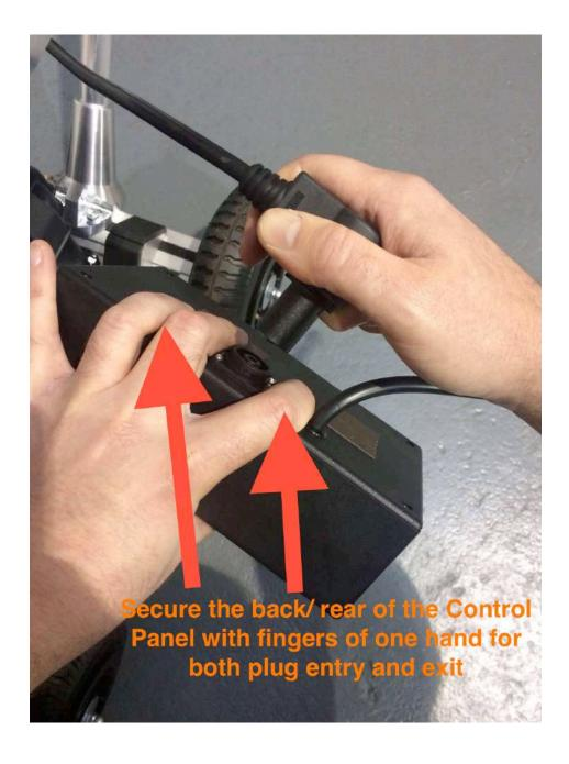
Always ensure that the correct plugs are placed into the correct sockets. Remember:
