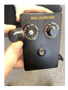
You can **rotate the Head section** of the machine left or right to a vertical position using the side handles pictured, you will be able to create top spin or back spin by increasing the speed of either wheel using the rotary dials on the Control Panel.
