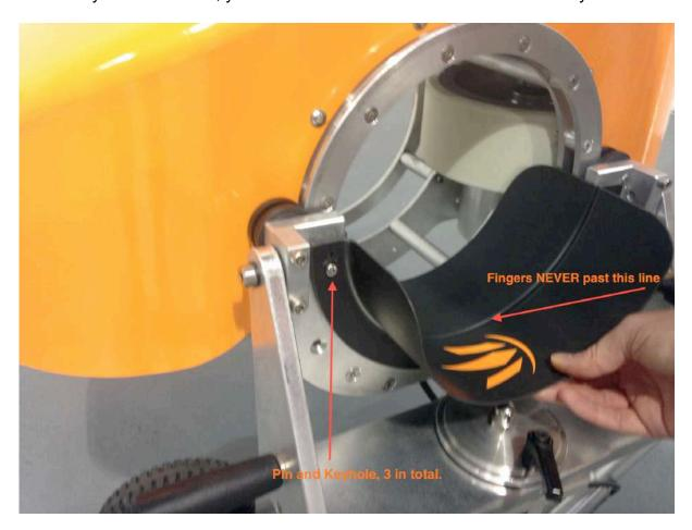
Take care when removing the Ball Feed from Ball Launcher, you must gently lift and then pull the Ball Feed away from the machine taking care not to damage the Ball Feed or the three pins on Trolley Frame section.
