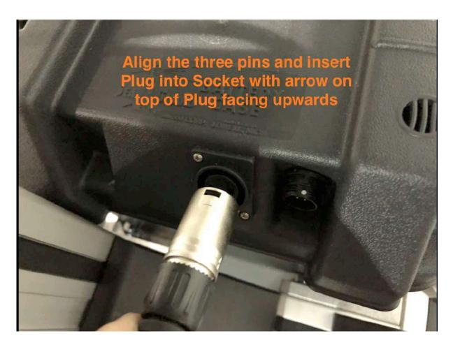
To remove cable on disassembly simply carefully pull the plug out.
