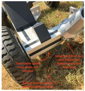
To operate, when in use and power is on move the induction lead to a position where the end of the lead is touching the ground and stays in contact with the ground. This has the effect of earthing any static charge generated by the machine and releasing it.
