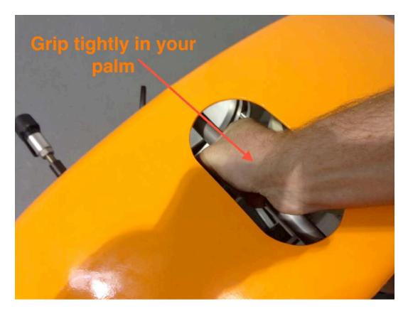
On the Trolley Frame section grip using both hands underneath.
