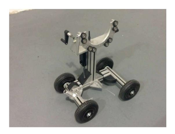
The dimensions of the Trolley Frame section are 66 cms height, 47 cms width and 66cms length.
