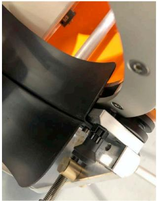
Below is the Plunger Pin in a fixed 'in' position where you can see that the Pin of the Plunger is inserted into the hole of the metal ring behind therefore fixing it into position.
