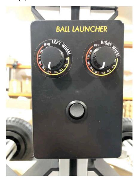
CURL, if the Head section of the Ball Launcher is placed in a horizontal position and the right wheel is placed on 60mph and the left wheel at 20mph, the football will exit the machine and curl to the left. The opposite effect will occur if the left firing wheel is placed on 60mph and the right wheel on 20mph and the football will curl to the right.
