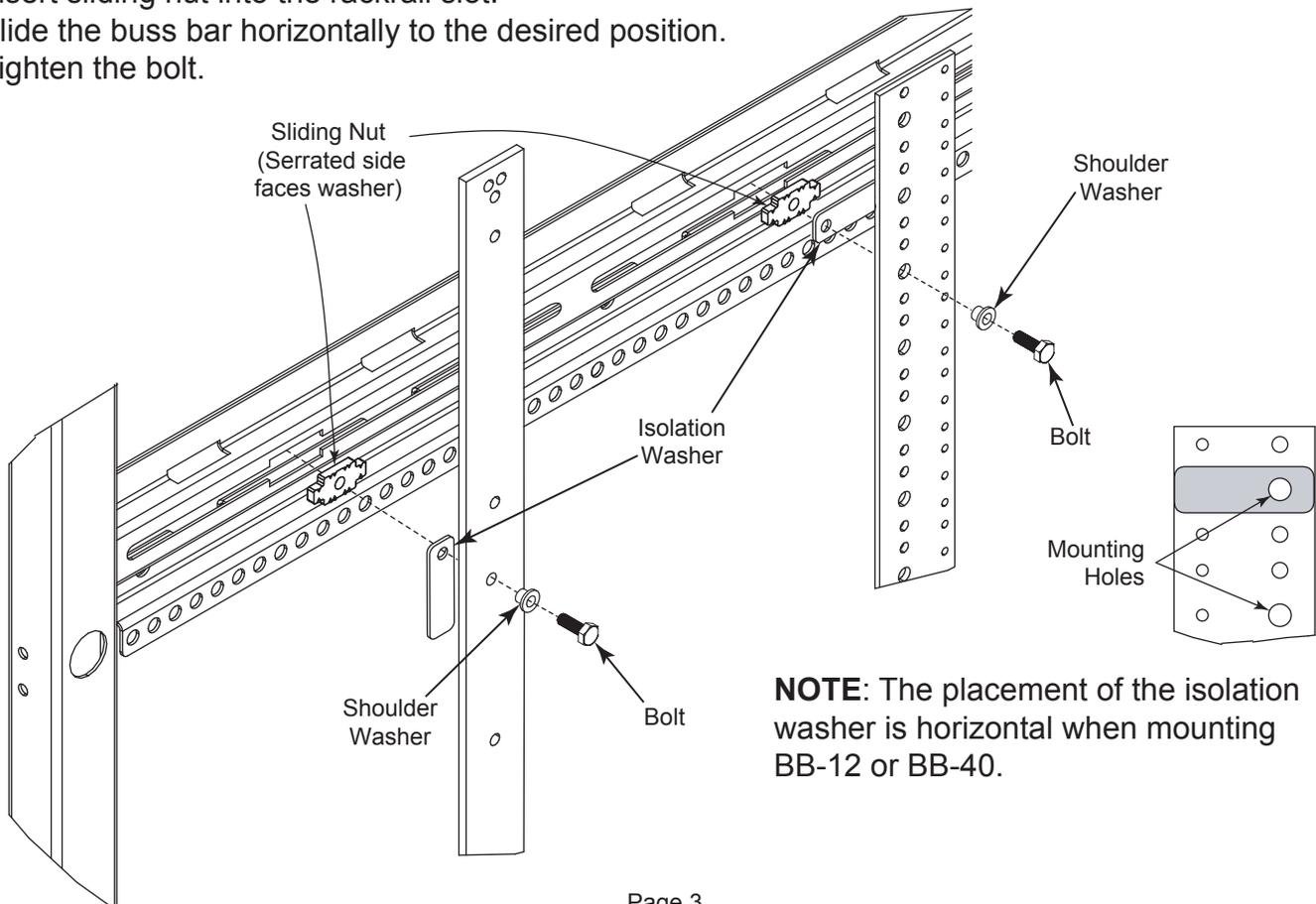
**NOTE:** The placement of the isolation washer is horizontal when mounting BB-12 or BB-40.
