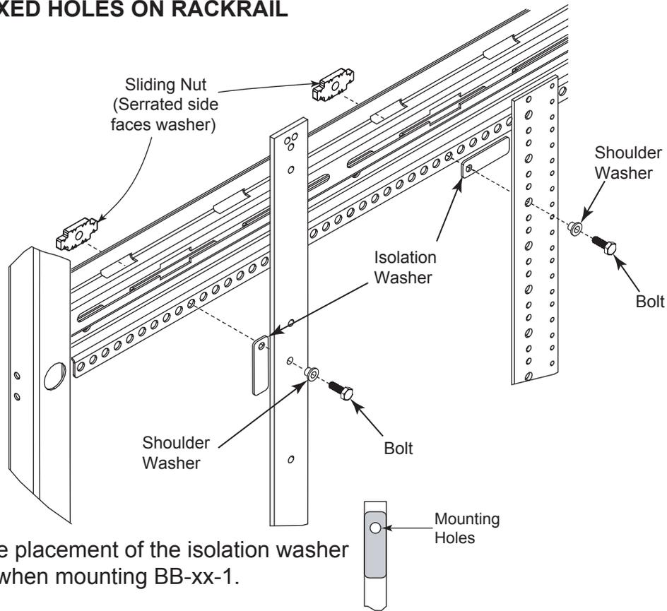
**NOTE:** The placement of the isolation washer is vertical when mounting BB-xx-1.
