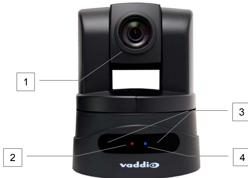
Figure 2: ClearVIEW HD-18 camera (front)
