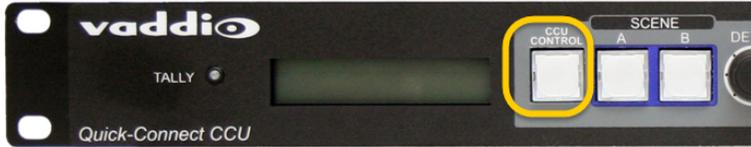
2. After booting, the display indicates the CCU is in Firmware Load mode.
