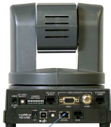
Connect to the Local Area Network or to a computer with a Cross-over cable
