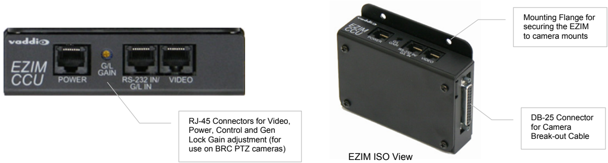
Figure 3: EZCamera Interface Module CCU (EZIM) with three (3) RJ-45 connectors for POWER, RS-232 IN / GEN LOCK and VIDEO, Top View (left) and Isometric View (right)
