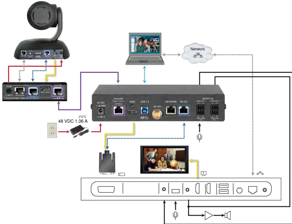
This diagram shows the camera and OneLINK HDMI extension connected to the codec and separately providing an IP video stream. It depicts the required Polycom fan-out cable and the signal types it carries. The OneLINK HDMI extension also provides IR forwarding.
