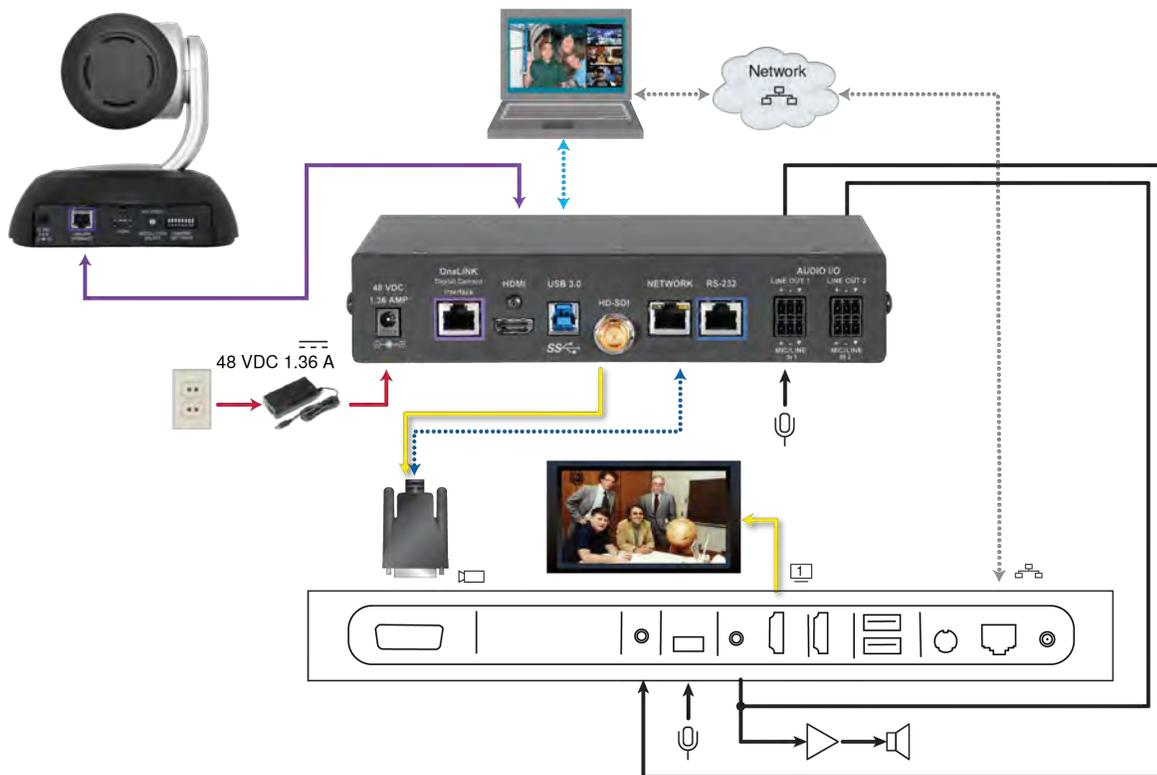
This diagram shows the camera and OneLINK HDMI extension connected to the codec and separately providing an IP video stream. It depicts the required Polycom fan-out cable and the signal types it carries. The OneLINK HDMI extension also provides IR forwarding.
