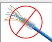
Please do not use “pass-thru” type RJ-45 connectors. These pass-thru type connectors do not work well for professional installations and can be the cause of intermittent connections which can result in the RS-232 control line failing and locking up, and/or compromising the HSDS™ signals. For best results please use standard RJ-45 connectors and test all cables for proper pin-outs prior to use and connection to Vaddio Cat-5e products.
