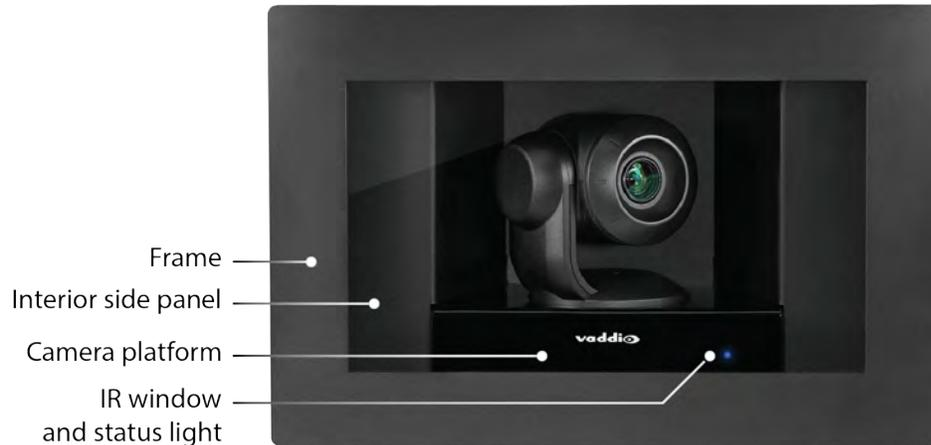
**Camera and Lens** – The 10x optical zoom lens and Exmor® 1/2.8 type, high-speed, low-noise image sensor deliver crisp full-HD video.
