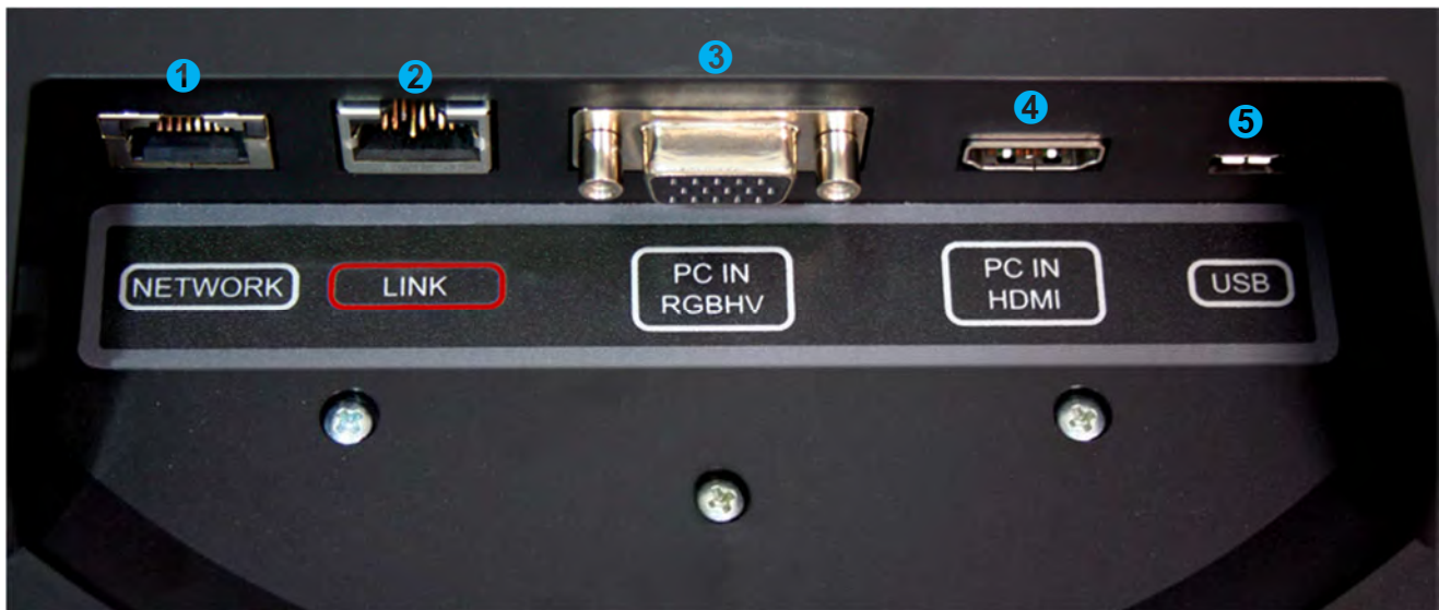
Image: BaseSTATION Dock Connector Panel Bottom View with Call-outs (BaseSTATION Dock turned over to read connector labels)
