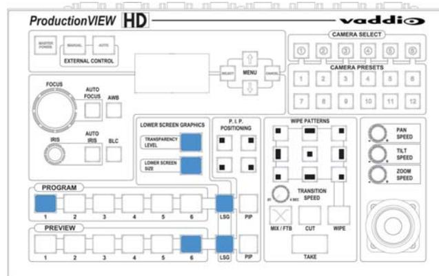
**Transparency Level:** To increase or decrease the transparency of the graphic overlay, press and hold the Transparency Level button down. The system will toggle through the levels to allow the user to select the level that is appropriate for the graphics.
