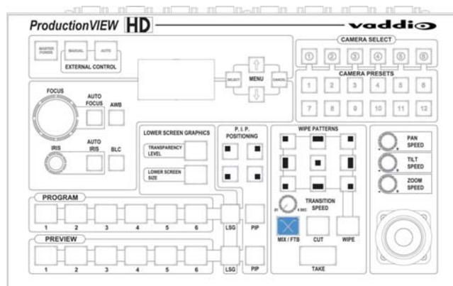
**FTB Speed:** The speed at which the signal fades in and out can be adjusted through the internal menu of ProductionVIEW HD. Speed ranges from 01 to 40 (.01 to 4.0 seconds). See the ProductionVIEW HD Menu Structure section of this manual for the location of the internal menu that adjusts FTB timing.
