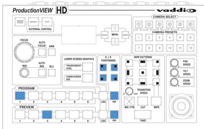
To display the PIP, press either of the PIP buttons, and the PIP will appear on the screen. Input 3 will now be displayed in a window in the lower left corner of the screen.
