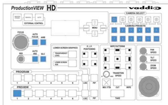
**3-Axis Joystick:** Within the menus, the 3-axis joystick is programmable for pan, tilt and zoom direction control. The zoom-in/zoom-out, tilt-up/tilt-down and pan-left/pan-right commands can be inverted on all 3-axis to customize control of the PTZ cameras attached to ProductionVIEW HD. Pan, Tilt and Zoom speed can be adjusted on controls above the joystick. The PTZ speeds are on a per-camera basis.
