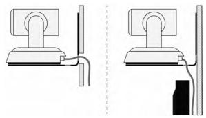
6. Attach the camera to the mount using the  $\frac{1}{4}$  -20 x .375 mounting screw supplied with the camera.
