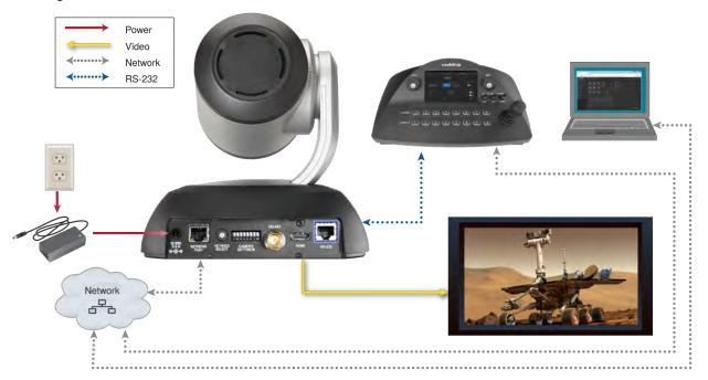
This example uses a PoE+ mid-span power injector, allowing the camera to be placed at a distance from the nearest power outlet.
