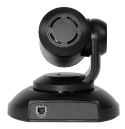
**Network/PoE+** – RJ-45 connector. Connect to a powered port on the PoE+ switch. It doesn't get much easier than that, does it?
