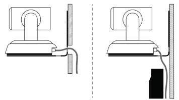
3. Attach the camera to the mount using the mounting screw supplied with the camera.
