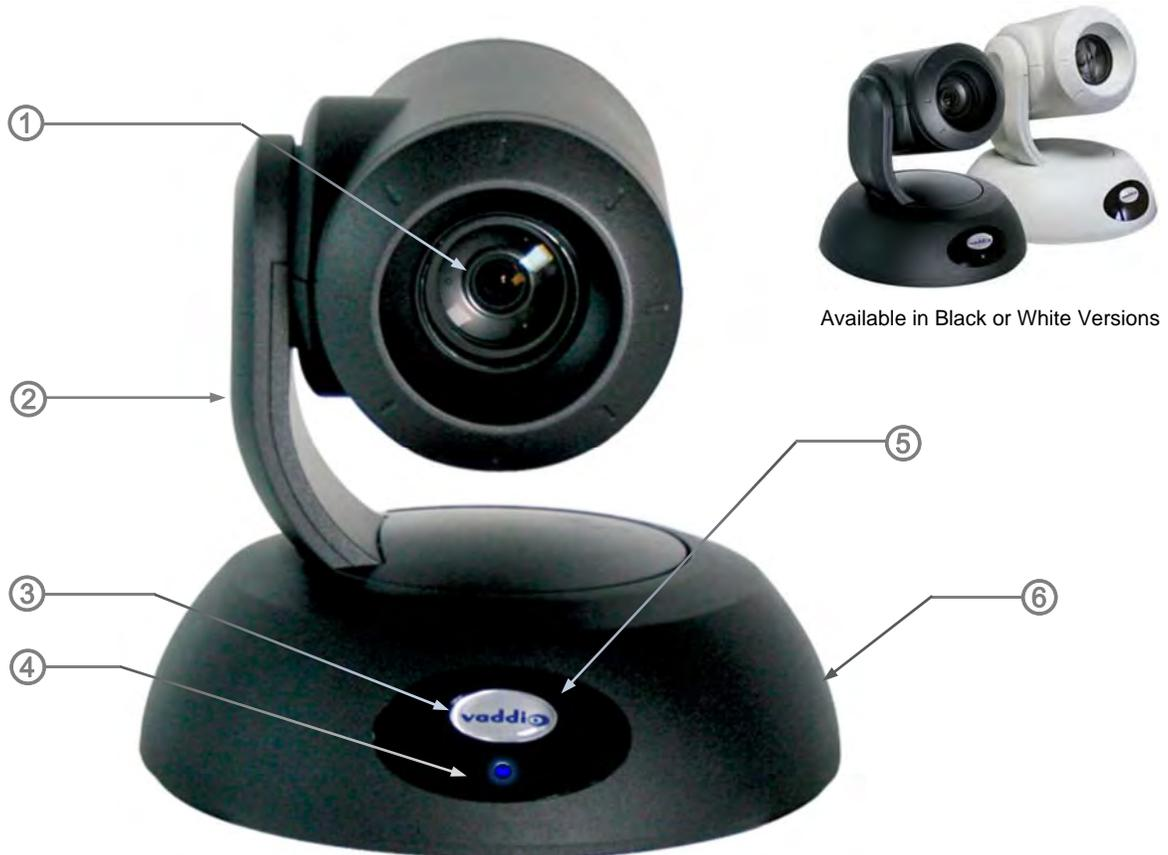
**1) Camera and Zoom Lens:** This RoboSHOT model has a powerful 30X optical zoom lens that is built around an Exmor 1/2.8-Typ, high-speed, low noise image sensor with a total of 2.38 megapixels (2.14 effective megapixels) for vibrant, detailed HD video image acquisition in a large to medium sized room.
