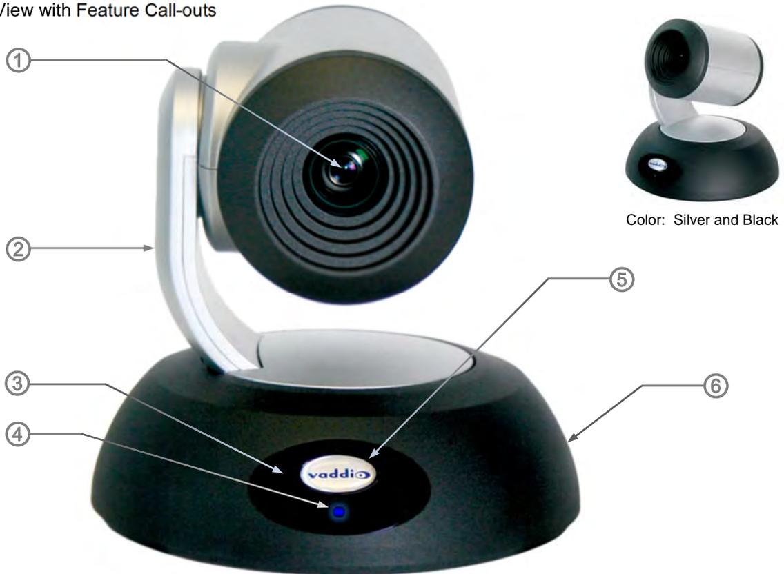
**1) Camera and Zoom Lens:** This RoboSHOT model features a 12X optical zoom lens (12X in Super-Wide mode and 10X in normal mode) that is built around an Exmor 1/2.8-Type, high-speed, low noise image sensor with a total of 2.38 megapixels (2.14 effective megapixels) for exceptionally precise HD video image acquisition in a small to medium sized conference room.
