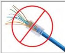
**Please do not use "pass-thru" type RJ-45 connectors. These pass-thru type connectors do not work well for professional installations and can be the cause of intermittent connections which can result in the RS-232 control line failing and locking up, and/or compromising the HSDS (high speed differential signals). For best results please use standard RJ-45 connectors and test all cables for proper pin-outs prior to use and connection to Vaddio Cat-5e products.**
