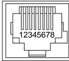
Pin # RJ-45 RS-232 and IR Out Pins
