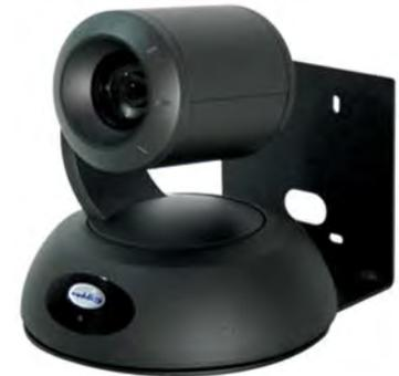
The mounting holes are slotted and are 90° opposing to provide easy leveling. Level the mount and place the camera on the mount. Connect the marked and tested Cat-5e cables to the appropriate RJ-45 jacks. Check the level again to avoid any of those weird Batman camera angles. Use the provided ¼”-20 x .375 mounting screw to attach the Camera to the mount.
