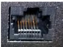
**Intact** – Contact fingers will make reliable contact with the cable connector
