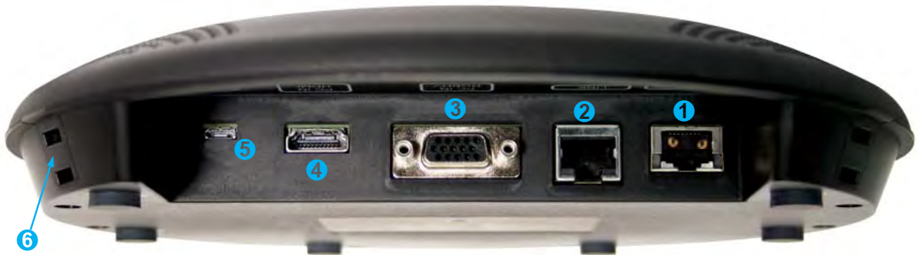
Image: Huddle Dock Connector Panel Bottom View with Call-outs (Dock turned over to read connector labels)
