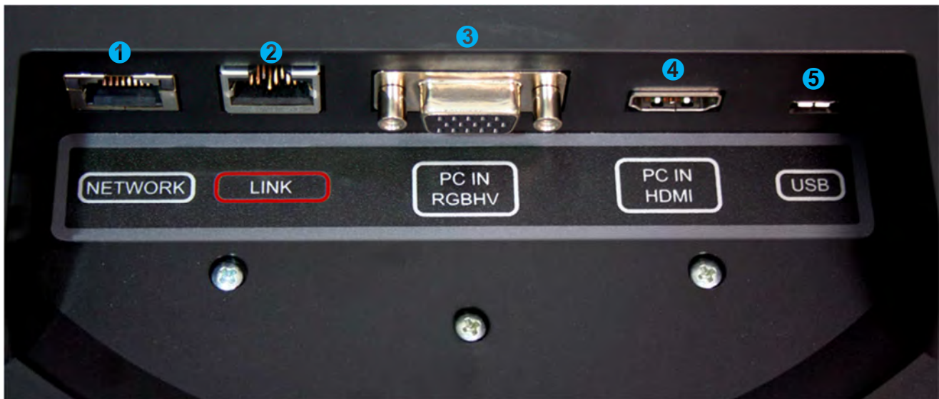
Image: Huddle Dock Connector Panel Bottom View with Call-outs (Dock turned over to read connector labels)
