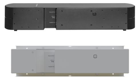
**Network/PoE+** – RJ-45 connector. Connect to the network and to power via the Power and Data Out port of the mid-span PoE+ power injector. Provides power and network access for IP streaming and camera control via web interface or Telnet.
