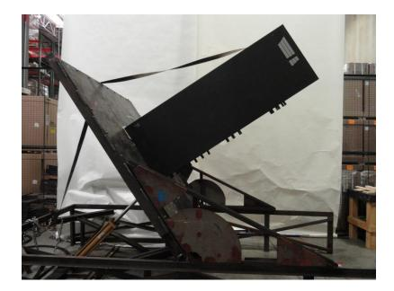
Photo 2 ERK-4428 at maximum inclination in front-to-back direction
