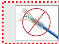
Please do not use "pass-thru" type RJ-45 connectors. These pass-thru type connectors do not work well for professional installations and can be the cause of intermittent connections which can result in the RS-232 control line failing and locking up, and/or compromising the HSDS™ signals. For best results please use standard RJ-45 connectors and test all cables for proper pin-outs prior to use and connection to Vaddio product.
