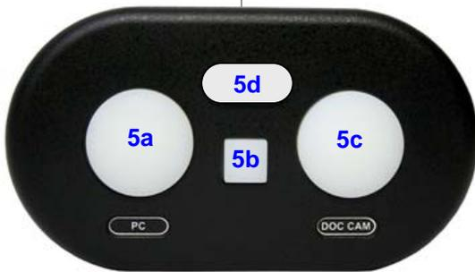
**PresenterPOD 1 (no scale):** Buttons marked to correspond to the icons on the Trigger Outs of PresenterPOD 1. The PresenterPOD is connected to the POD 1 Interface with a Cat-5e cable (up to 100' /30.48m).
