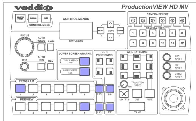
**Transparency Level:** To increase or decrease the transparency of the graphic overlay, press and hold the Transparency Level button down. The system will toggle through the levels to allow the user to select the level that is appropriate for the graphics.
