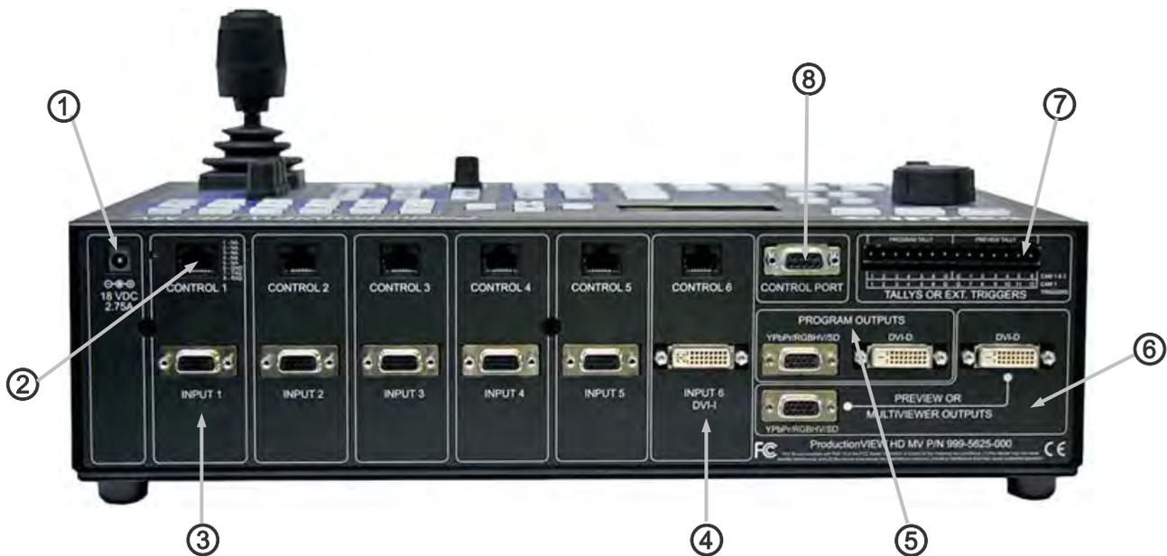
1. **Power Input:** Use only the 18 VDC, 2.75A power supply provided with the ProductionVIEW HD MV.
