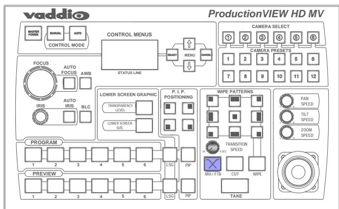
**FTB Speed:** The speed at which the signal fades in and out can be adjusted through the internal menu of ProductionVIEW HD MV. Speed ranges from 0.1 to 4.0 seconds (01 to 40 in the menu). See the ProductionVIEW HD MV Menu Structure section of this manual for the location of the internal menu that adjusts FTB timing.
