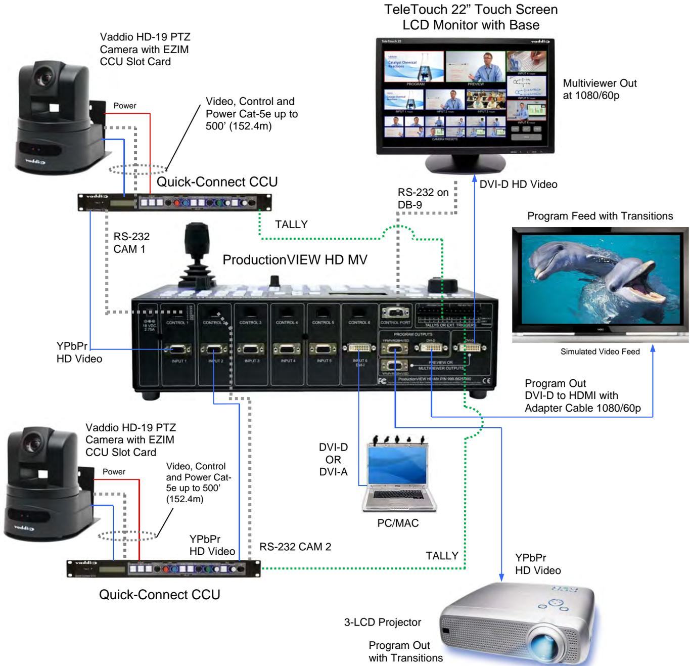
**ProductionVIEW HD-MV with Dual Bus mode connected to four-HD-20 PTZ Cameras, a TeleTouch 22” Touch Screen Controller and a standard YPbPr Monitor:**
