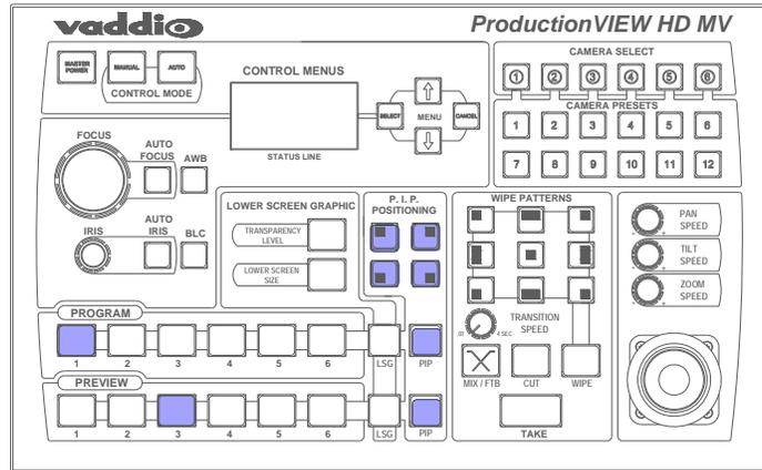
To display the PIP, press either of the PIP buttons, and the PIP will appear on the screen. Input 3 will now be displayed in a window in the lower left corner of the screen.
