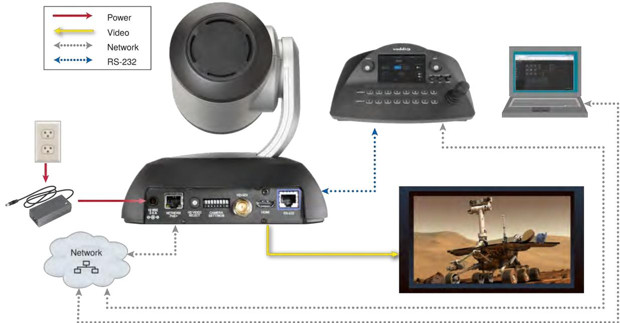
This example uses a PoE+ mid-span power injector, allowing the camera to be placed at a distance from the nearest power outlet.
