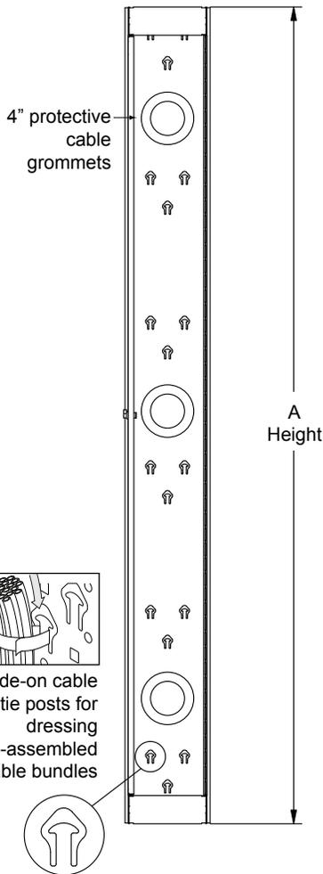
Removable panels allow for easy installation of existing cable bundles
