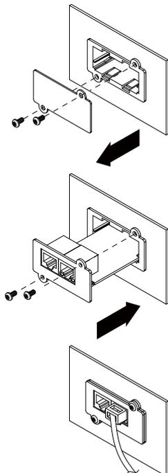
**NOTE:** The Middle Atlantic UPS-OLIPCARD is hot-swappable, so you do not need to turn off the device to install it.
