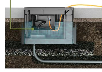
66 We needed to test the box to see if it worked well in all conditions, and we tested with about **53** inches of water
