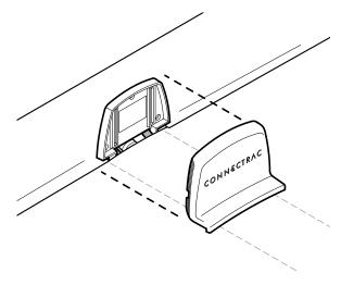
Use mounting tape to stick the backplate against the wall base, making sure to align the legs in the aluminum bottom track.
