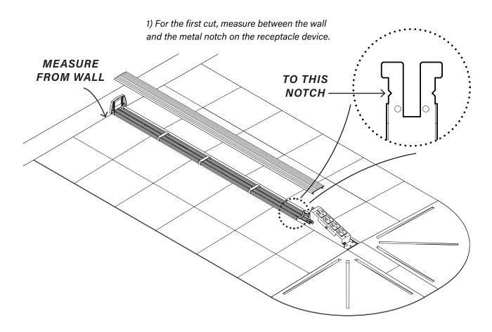
2) For the second cut, measure from the end of the wireway to the end of the device (minimum length 2"). Then snap those top cap pieces into your wireway.
