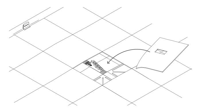
For the carpet tile covering the device, measure from the carpet to the edge of the device on two sides: Then transfer those measurements to your carpet and cut a hole for the device:
