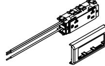
**Duplex Receptacle** – 3-wire, 20A, 125V, NEMA 5-20R. Provided with 10 1/2" (267mm) pigtails and inline splice connectors.
