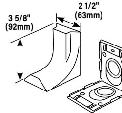
**FiberReady Transition Feed Fitting** – Eliminates offsetting V2400 in connecting with surface panel boxes. Has 3/4" and 1" concentric trade size KOs with 1" trade size KO elongated so adjustment from surface to center of bushing is 1" (25mm) minimum to 1 5/8" (41mm) maximum. Has twistouts for transition to Pancake 1500 and 2600 Series Raceway.
