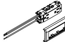
**Isolated Ground Duplex Receptacle** – 3-wire, 15A, 125V NEMA 5-15R. Provided with 10 1/2" (267mm) pigtails and inline splice connectors.
