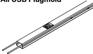
Available in 3' [914mm], and 5' [1.5m] lengths with 12" spacing. USB is 2.4 Amps (shared between two ports) 5VDC. .040" [1.0mm] steel housing. Packed two per carton. Each unit supplied with one (1) Coupling and two (2) Blank End Fittings. Each USB module provides 2 ports with 2.4 Amps of shared charging. Please note the charging load on one module will not affect the charging performance of the other USB modules in the product.
