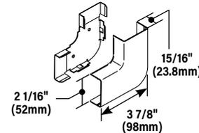
**90° Flat Elbow –** For right angle turns on the same surface (nonmetallic cover).
