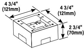
**Extra Deep Device Box** – Base has rectangular knockout to enable extension from existing single-gang flush wall box and 1/2" and 1" concentric KOs. Cover has twistouts for 500/700 Series Raceway on each end and twistouts for 2400 Series Raceway on each side.
