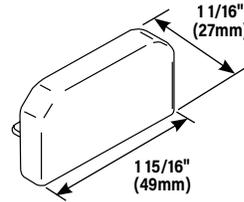
**Blank End Fitting** – Use with NM2000 Series.
