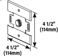
**Back Feed Fitting –** For feeding 2400 Series Raceway from an existing outlet box. Equipped with 1/2" trade size male bushing and locknut washer for grounding.
