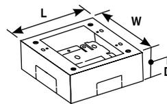
**Device Box –** Base has 1/2" trade size KO and rectangular KO for extension to wall box. Has #10 threaded hole for ground connection. Cover has twistouts for 500/700 Series Raceway on each end and twistouts for 2400 Series Raceway on each side.
