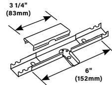
**Side Reducing Connector** - connects 2000 Series Plugmold with 500 Series Raceway through the side of 2000 Series Plugmold.
