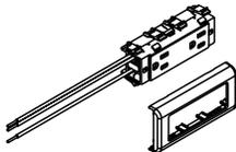
**Duplex Receptacle** – 3-wire, 15A, 125V, NEMA 5-15R. Provided with 10 1/2" (267mm) pigtails and inline splice connectors.
