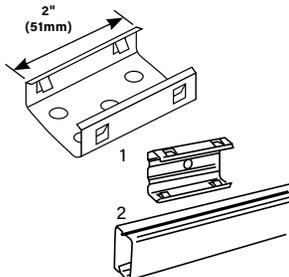
**2003 Supporting Clip -** Temporary support, while positioning lengths of raceway base. Use with 2000 Series Raceway.
