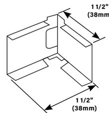
**Internal Corner Coupling** - Furnished with one fiber bushing.
