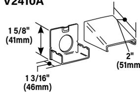
**Entrance End –** For connecting V2400 with 1/2" trade size conduit and armored cable. Use with V2400 Series Raceway.
