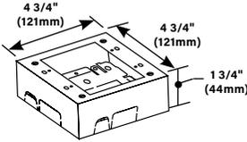
**Two-Gang Device Box** - Cover has twistouts for 2000, 500 and 700 Series Raceways. Base has 1/2" trade size KO and rectangular KO for extension to wall box. Base has No.10 threaded hole for ground connection.
