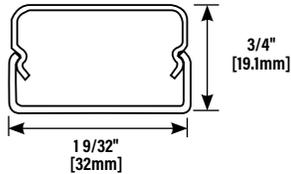
Available in 3' [914mm], 5' [1.5m] and 6' [1.8m] lengths with 6" [152mm] receptacle spacing. 15A tamper-resistant receptacles. 3-wire, #12 THHN (1 hot, 1 neutral, and insulated ground conductor rated for use on 20A circuits). .040" [1.0mm] steel housing. Packed 2 per carton. Each unit supplied with one (1) Coupling and two (2) Blank End Fittings. USB is 2.4 Amp (shared between 2 ports) 5VDC.
