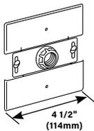
**Flush Plate Adapter** - Feeds 2000 Series Plugmold from an existing wall outlet. Equipped with 1/2" (12.7mm) threaded stud, toothed lock washer for grounding, threaded hole for and conduit bushing.
