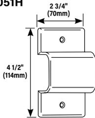
**Wall Box Adapter** – For feeding raceway from an existing wall outlet; horizontal applications. Provides complete access to wall box for connections.
