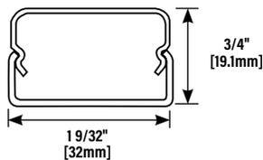
Available in 5' [1.5m] length with 9" spacing. 15A tamper-resistant receptacles. 3-wire, #12 THHN (1 hot, 1 neutral, and insulated ground conductor rated for use on 20A circuits). .040" [1.0 mm] steel housing. Packed two per carton. Each unit supplied with one (1) Coupling and two (2) Blank End Fittings. USB is 2.4 Amps (shared between two ports) 5VDC. Please note the charging load on one module will not affect the charging performance of the other USB modules in the product.
